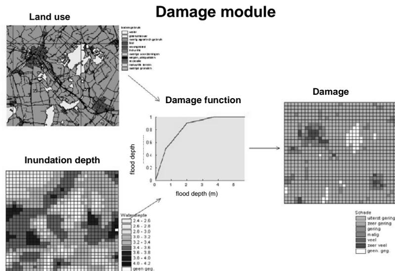
Figure 4: Principle of the method for assessment of economic damage
