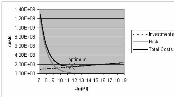
Figure 3: Relation between total costs and decreasing failure probability, for the example and corresponding variables analysed in (van Danzig, 1956):  $I_0 = 3.9 \cdot 10^7$  (Dfl),  $I' = 0.33 \cdot 10^6$  (Dfl),  $D = 24 \cdot 10^9$  (Dfl),  $r' = 0.015$  (/yr), 1 Euro = 2.2 Dfl)
