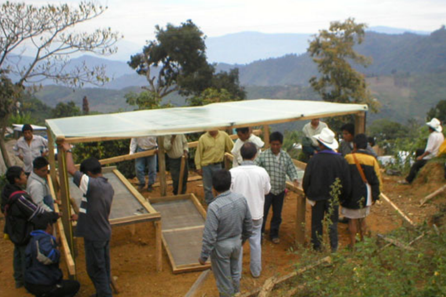
The solar coffee dryer is made from locally available wood and plastic. The trays are made from wood and steel mesh.
