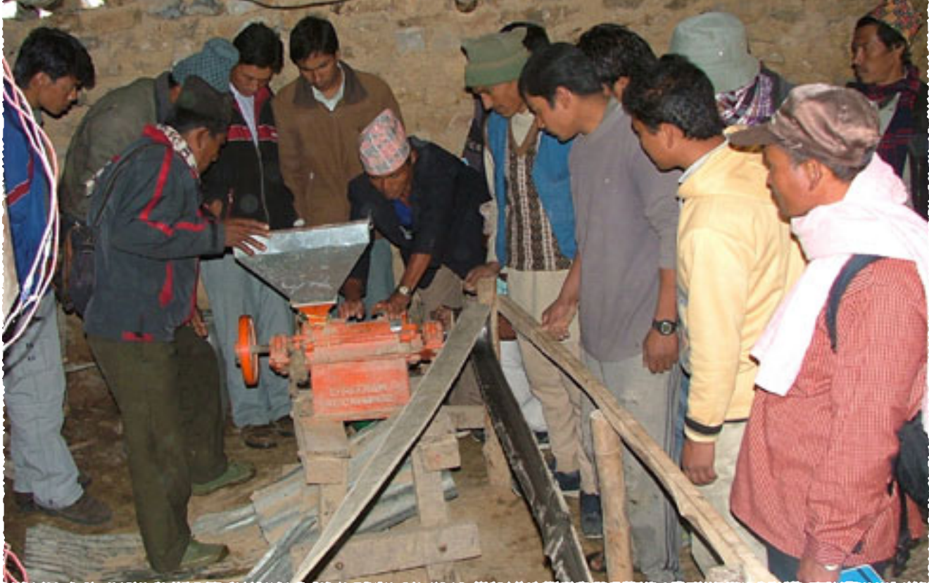
Installation of a paddy huller.
