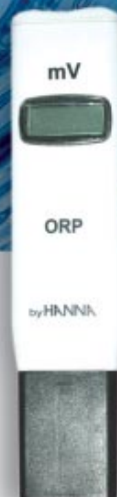
Figure 1 - A typical hand-held ORP meter.
