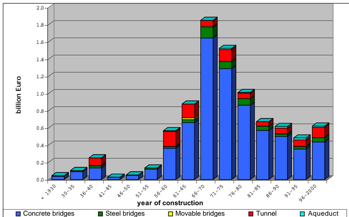
**FIGURE 2 Replacement value of structures related to years of construction.**
