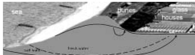
Figure 5: Restoration of water table and upward seepage in inner dune belt after stopping drinking water extraction in the dunes
