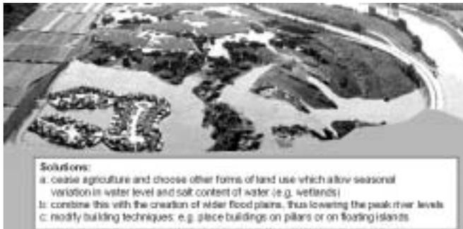
Figure 11: Expansion of wetlands/flood plains as a sustainable solution to stop further land subsidence and to avoid flooding of the rivers in view of climatic changes
