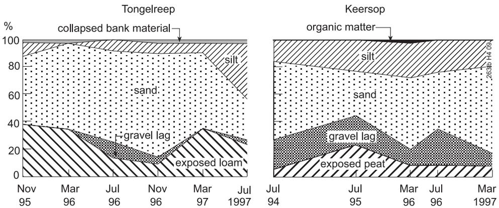
Fig. 4.9. Differences and changes in bed material
