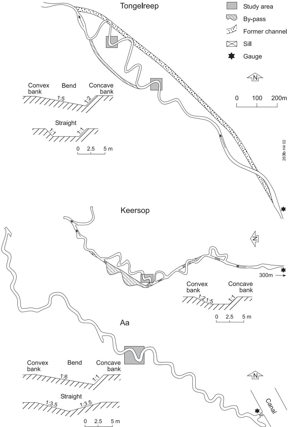
Fig. 4.2. Layout of the rehabilitation reaches, dimensions of cross sections excavated and the locations of the study sites
