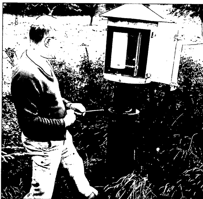
Figure 4.18 Automatic recorder mounted in an alternative instrument shelter (Belgium).
