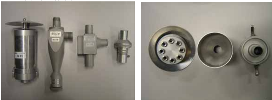
Figure 7.2 The left picture shows the air inlet head, the PM10 cyclone pre-separator, the PM2.5 cyclone pre-separator and the filter holder (from left to right) ; the right picture shows the construction of the air inlet head.
