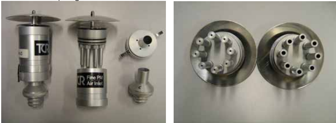
Figure 7.1 The left picture shows the complete sampling head; the right picture shows the difference between the size of the openings of the air pipes above the impaction plate (bigger openings for PM10; smaller openings for PM2.5)
