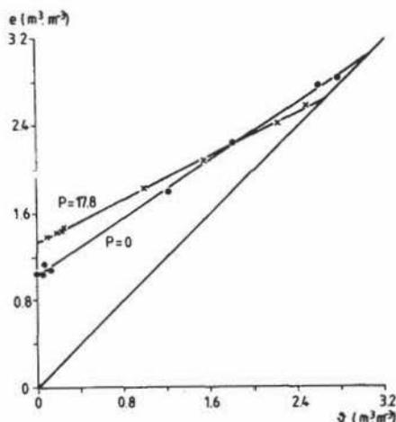
Fig. 8. The shrinkage characteristics of margalite clay as calculated from Fig. 6 and 7.
