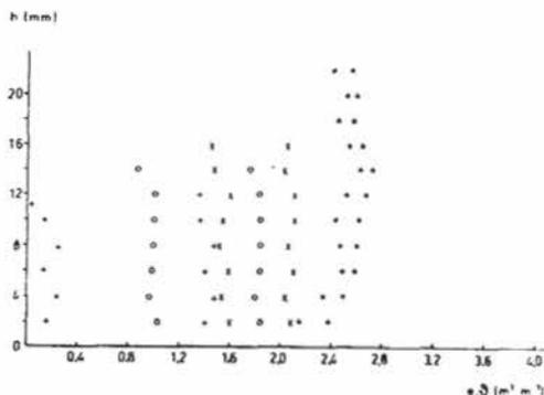
Fig. 6. Drying of an unloaded margalite clay. Points for  $v$  are on the right of those for  $e$ .
