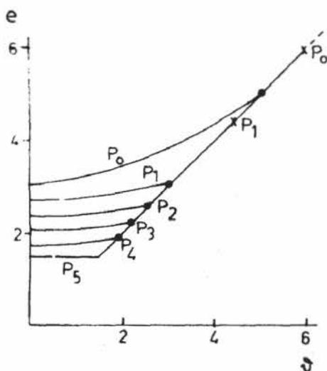
Fig. 3. Hypothetical shrinkage characteristic.  $\bullet$ — $\times$ : Part of curve, for constant  $P$ , where normal shrinkage prevails.  $P=0$  is indicated as  $P_0$ .
