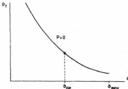
Fig.1 The Moisture Characteristic of a heavy clay soil.  $v$  is the moisture ratio ( $m^3$  water per  $m^3$  solid phase),  $p_t$  is the tensiometer pressure (Pa).
