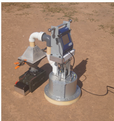
Fig. 6. a) PI-SWRL with dust recovery system, b) supply-limited surface with limited emissivity, c) not supply-limited, highly emissive surface.
