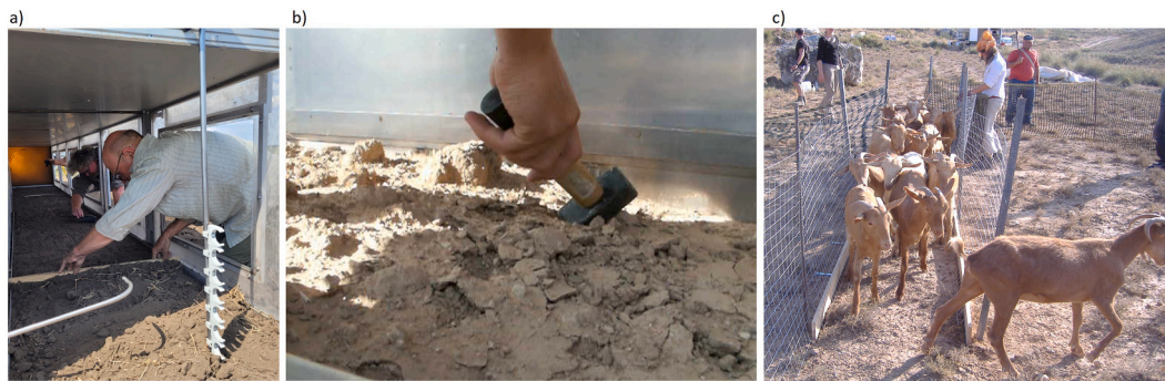
Fig. 7. Preparation of surface: a) levelling and reducing roughness for comparable surface, b) use of hammer to simulate hoof impact, c) animals led over the test plot prior to mounting the tunnel.
