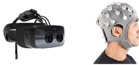
Fig. 1. Varjo XR3 headset and Enobio's 32 channel EEG system.
