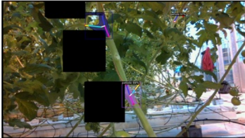
Fig. 4. To test the impact of occlusion on planner performance, more occlusion was simulated by adding black boxes in front of the plant nodes. The figure shows the rendered boxes in the camera image.
