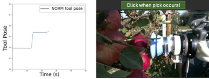
Fig. 5. User Interface for determining moment of abscission. The user was provided a video of the pick ( right ), as well as the z-position of the gripper ( left ), and was given a button to press when the pick occurred. The force signals were not provided to the subject.
