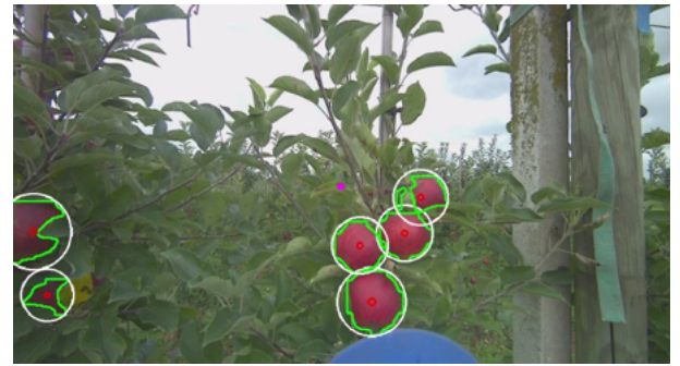
Fig. 4. Camera image with result of apple detection. Shown are the detected apple instances (green contour), enclosing circle (white circle), and region used for distance measurement (small red circle inside white circle)
