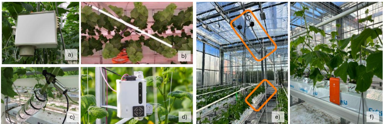
Figure 2.2 Each compartment was equipped with: climate measuring boxes for measuring temperature, relative humidity and CO 2 concentration (a); PAR sensors (b); sap flow and stem diameter sensor (c); camera's for vision technology (d); weighing gutters for measuring crop transpirations and fresh weight growth of the crop (e); slab sensors to measure EC, volumetric water content and temperature of the root-zone environment (f).
