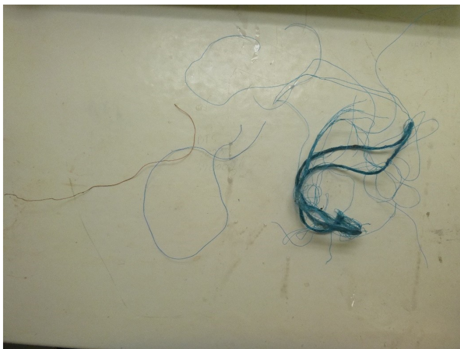
Photo 2 Example of "A7 – Synthetic rope" which is degrading into multiple "A5 – Monofilament" items, colour and length of the blue monofilaments clearly indicate they are originating from the blue piece of "A7 – Synthetic rope". Such a piece of synthetic rope can easily fall apart once in the cod-end together with the rest of the (fish and benthos) catch. The Dutch surveyors counted this catch of marine litter as one orange "A5 – Monofilament" and one blue "A7 – Synthetic rope".
