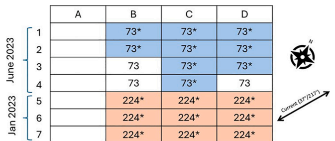
Fig. 2. Schematic overview of the solar farm layout during the time of sampling (September 2023). The numbers in the centre indicate the number of days that the floaters were in the water on the day of the sampling, and if a floater has an asterisk (*) then it was sampled. Floaters of column A were excluded from the sampling. The arrow indicates the current direction in relevance to the floater deployment.
