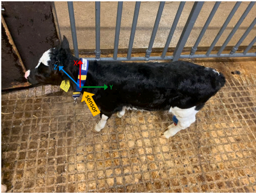
Fig. 3. The collar used to attach the accelerometer sensor and the orientation of the three axes. The X -axis detected the top-bottom direction, the Y -axis detected the backwards-forward direction, and the Z -axis detected the left-right direction.
