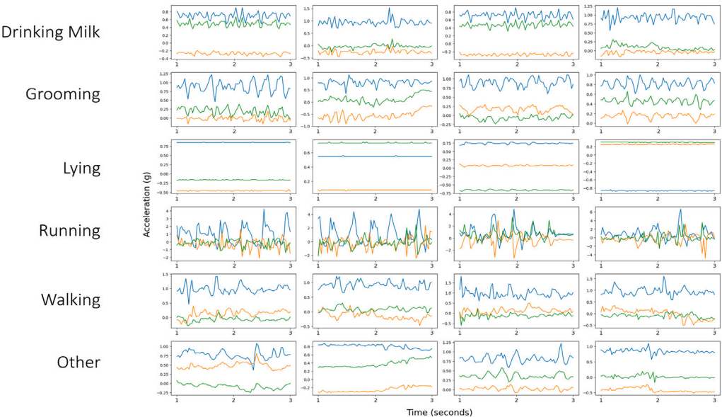
Fig. 8. Random 3 s time-windows selected from a set of random calves for each behaviour. Drinking milk and grooming behaviour have a subtle shape in the time-domain that is almost phase-aligned.
