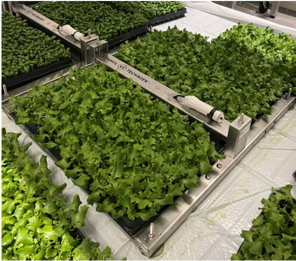
Figure 17 Tray weight sensor used in an experiment during lettuce and basil propagation phase
