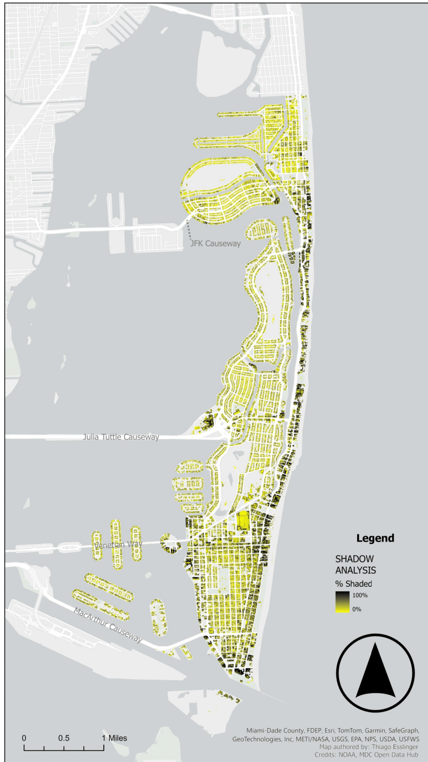
Figure 13. Shadow analysis for biosolar-suitable rooftops.
