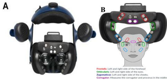
Figure 2: A) EmteqPRO inserts are mounted onto HTV pro B) Mapping between EmteqPRO sensors and facial muscles (adapted from Gnacek et al., (2021) [10]).
