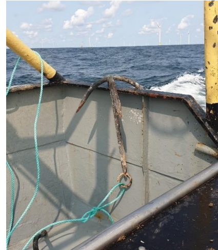
Figure A3.2 10/05/2024 light dredge anchor used for recovery of gill nets without markings.
