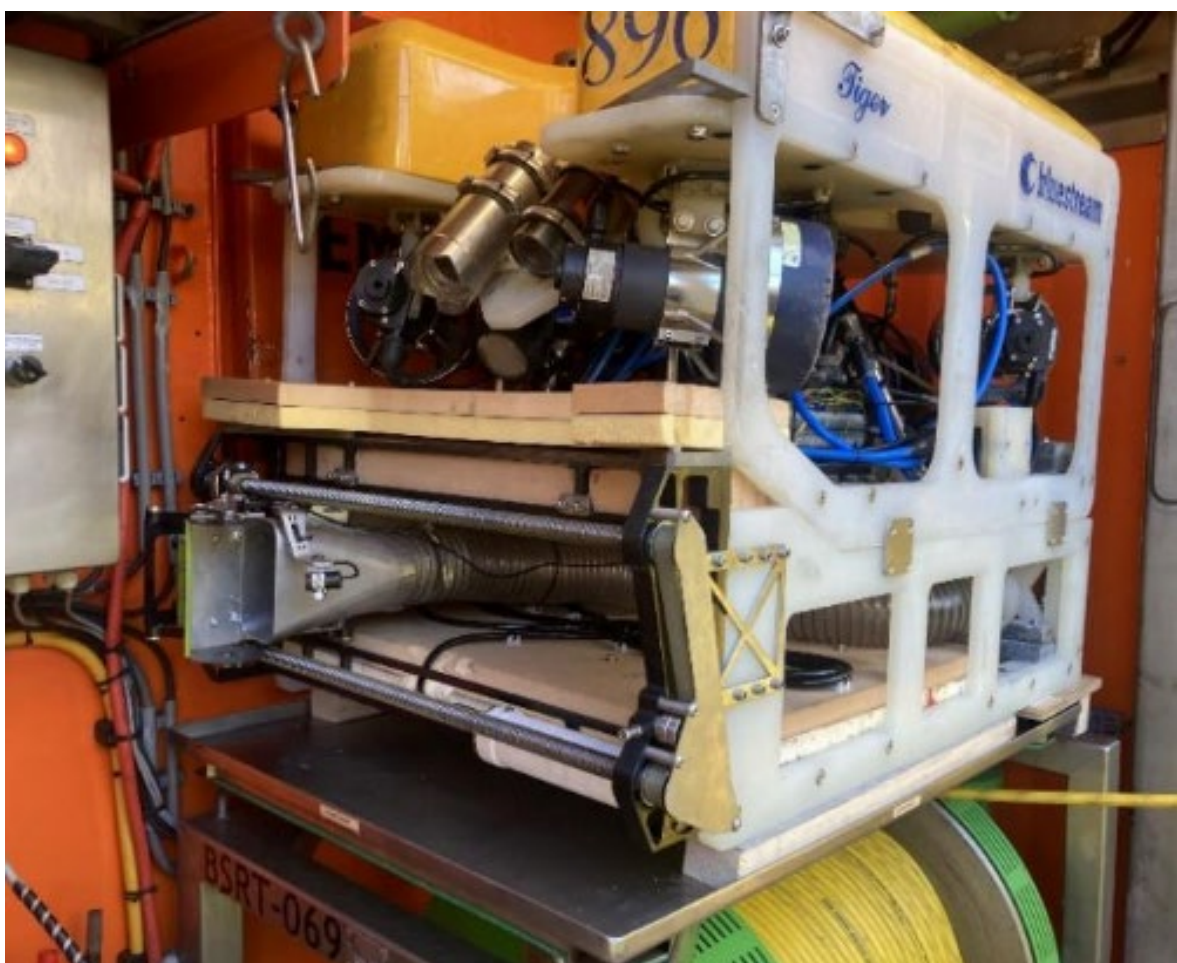
Figure 14. MGST mounted under the Saab SeaEye Tiger ROV (Coolen et al., 2024).
