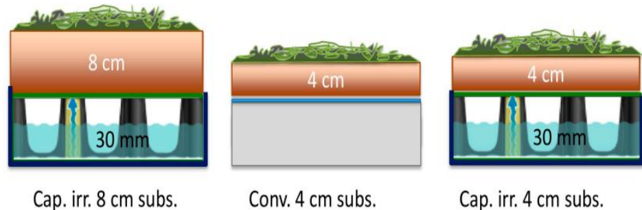
Figure 2. Schematic cross-sections of the three research plots. The left and right plot are equipped with the Permavoid drainage and capillary irrigation system.
