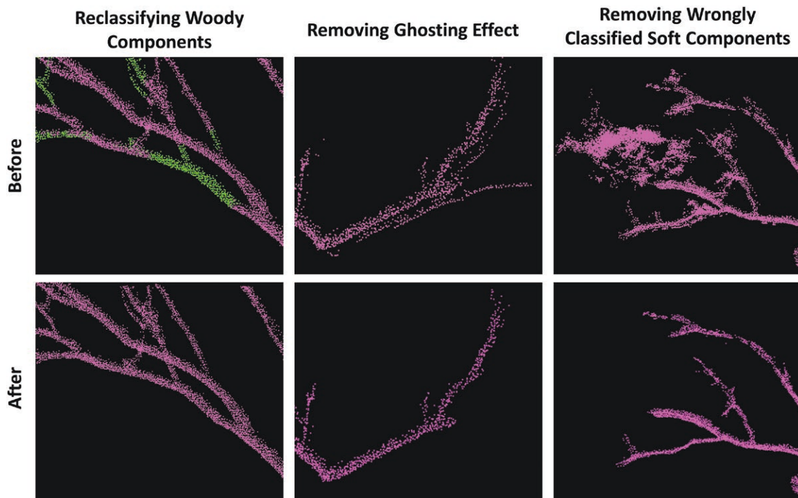
Figure 1. Examples of manual corrections made in the points clouds to adjust for errors in the LiDAR data and the output of the classification algorithm LeWoS (D. Wang et al. , 2020). Woody components are shown in purple and soft components in green.
