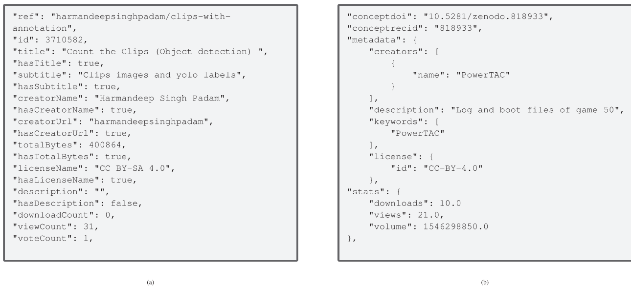
FIGURE 3 | Different metadata schemas utilized by different dataset hosting platforms. (a) Dataset metadata example from Kaggle. Source: https://www.kaggle.com/datasets/harmanDeepsinghpadam/clips-with-annotation . (b) Dataset metadata example from Zenodo. Source: https://zenodo.org/records/818934 .
