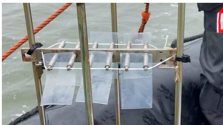
Figure 1.1 Picture of a set of six polydimethylsiloxane (PDMS) samplers that were used within this present study
