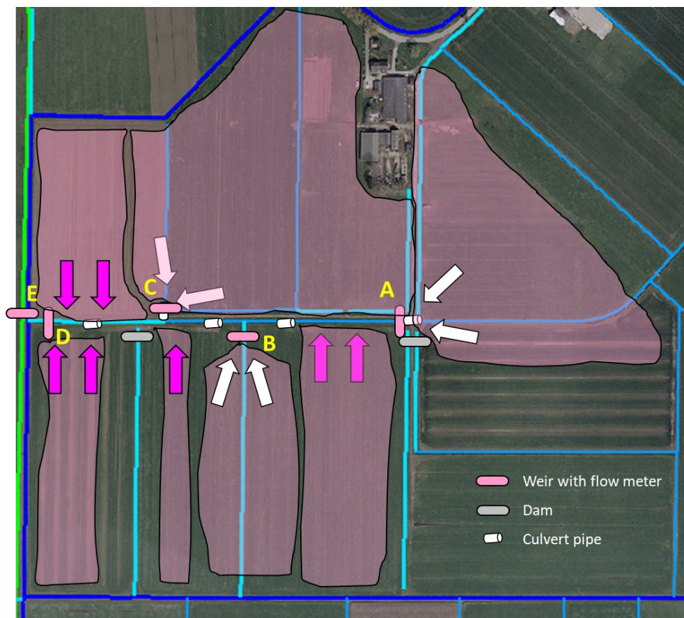
Figure 25 Position of five flow meters in the field study indicated by capital letters A to E. The watercourse between A and E is fed by direct runoff via trenches (purple arrows) and via drainage (pink-greyish area with white arrows).
