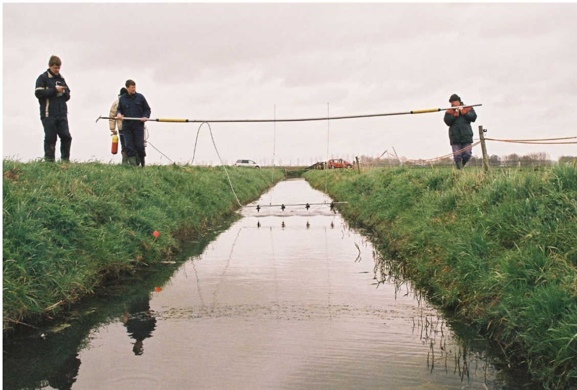
Figure 7 Spraying the application stretch of the ditch.
