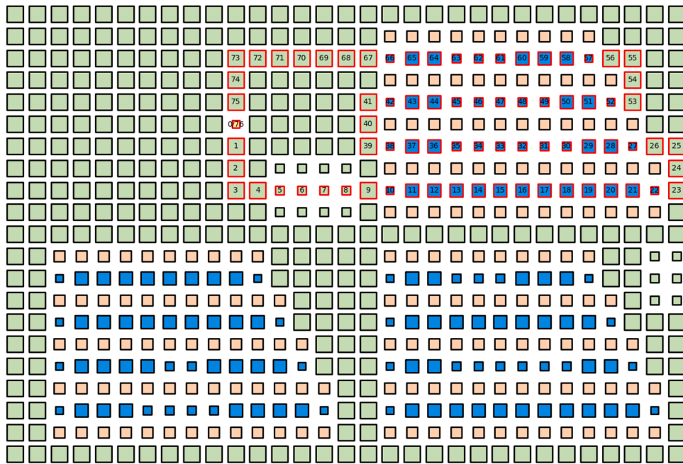
Fig. 11. Third case: Tractor 2 – Path inside the field, intuitively followed by a farmer, the numbers in the cells represent the steps the farmer would follow in the field.
