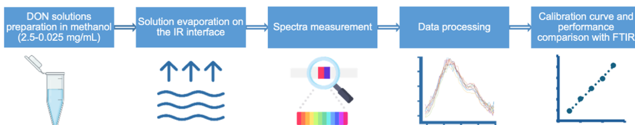
FIG. 3. Analytical workflow, including sample application, measurement, and data processing workflow for the comparative evaluation of the IR devices.
