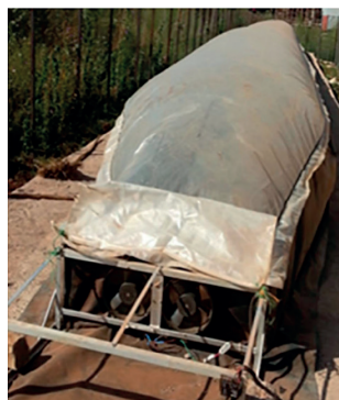
Figure 2.3. Solar bubble drier (photo with permission from GrainPro®; (Asemu et al. , 2020)). (Asemu et al. , 2019)
