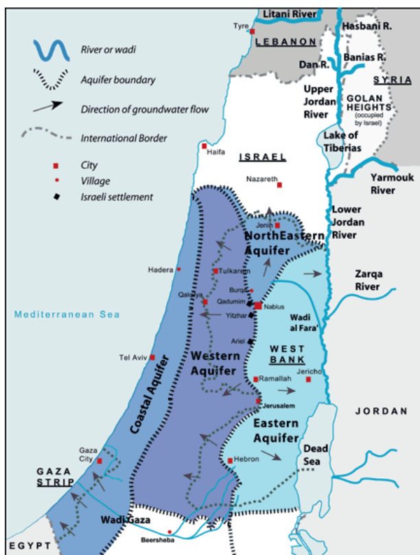
Figure 4.1 Basin formations and directions of groundwater flows
