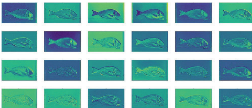
Figure 2.9 Extracted features by each convolutional block for visceral weight prediction. The four rows represent the four convolutional blocks shown in the NN architecture. Each row only contains features obtained from the layers in the same block.
