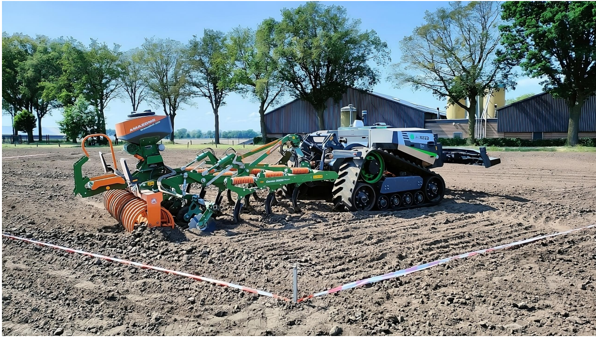
Figure 4.1: The AgBot 5.115T2 of the company AgXeed B.V (The Netherlands) with a mounted Amazone Cenius 3000 Super cultivator combined with a seed drill.
