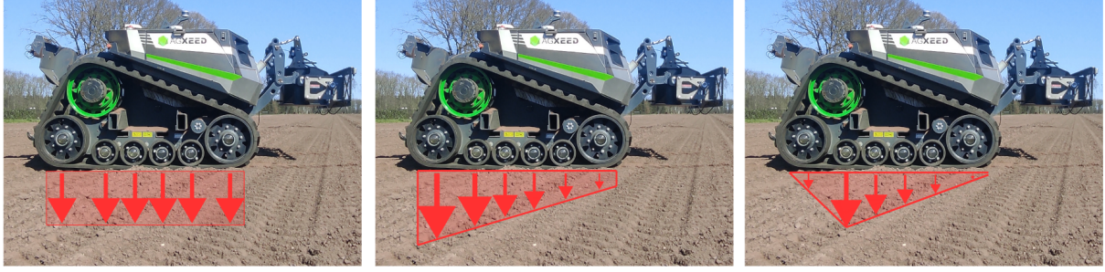
Figure 5.2: Load distribution on tracks according to Uniform, trapezoidal and triangular distributions
