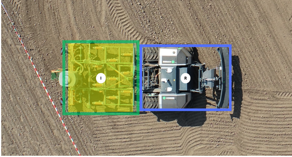
Figure 4.3: Autonomous robot, represented by a blue box, equipped with a mounted implement, indicated by a green box. The coverage area of the implement is highlighted in yellow. The centers of both the robot and the implement are marked with symbols 'R' (for robot) and 'I' (for implement), respectively.
