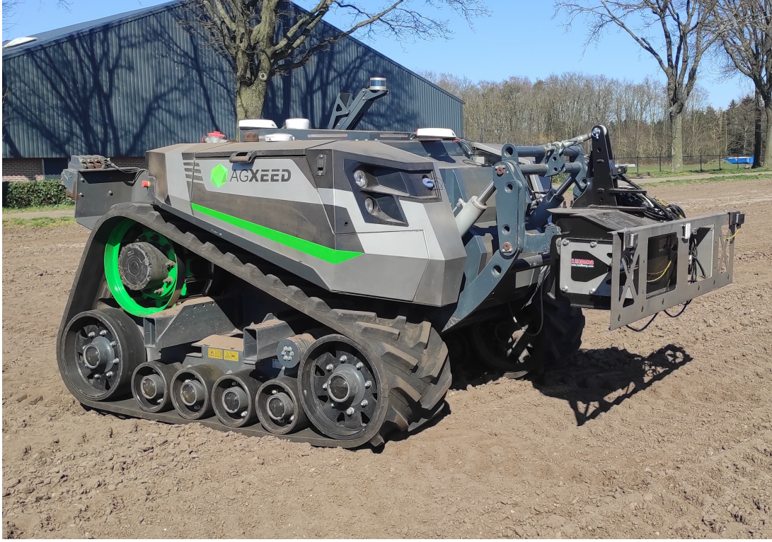
Figure 2.2: The AgBot 5.115T2, from the company Agreed B.V (The Netherlands), is a differential robot with continuous treads. The weight of the robot is 7.8t, the total width of the robot is 2.5 m, the minimum turning radius avoiding excessive soil damage is 2.1 m. For the experiments, the operational width of the robot (width of the coupled tool) was assigned the same value as the width of the robot. The AgBot 5.115T2 has 4-cylinder Deutz Diesel Engine, stage 5 with 156hp, and an electric drive train with a maximum speed of 13.5 km/h. Some onboard sensors are 2 cameras, a RTK-GNSS receiver and an IMU.
