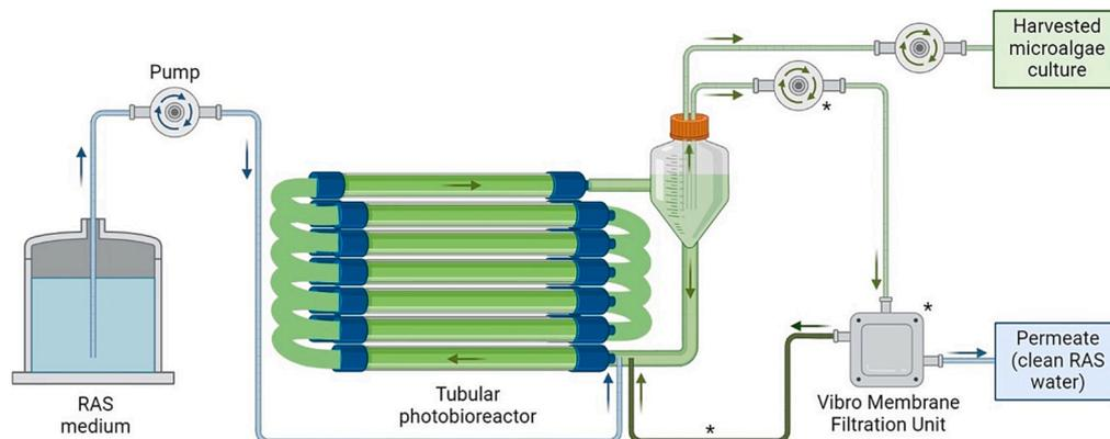
**Fig. 1.** Schematic drawing of the reactor setup for perfusion cultivation and continuous cultivation mode (asterisks indicate flows/equipment belonging to the membrane filtration that is only used for perfusion mode).
