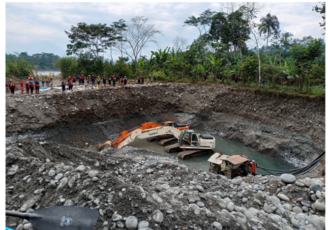
Fig. 4. Impact caused by mining activities (hole made by backhoe). Inspection carried out in Jatun.
