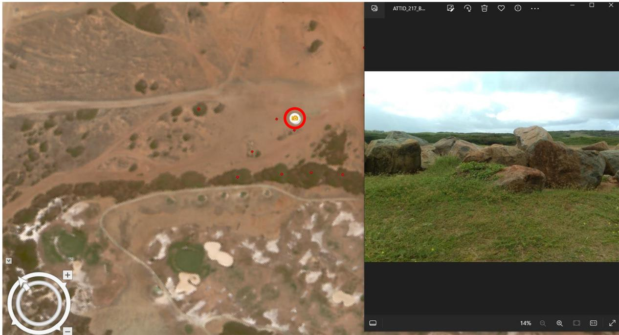
**Figure 6** Difference in acquisition time and phenology between the field survey (November 2022) and the image acquisition date (May 2020) might have caused some problems in the image classification. May 2020 was a very dry month as can be seen in the WV-3 image, while the field survey was conducted after heavy rains that caused the vegetation to bloom. The mixed grass cover shown in the photograph (right) displays lush growth, whereas the satellite image shows bare soil.
