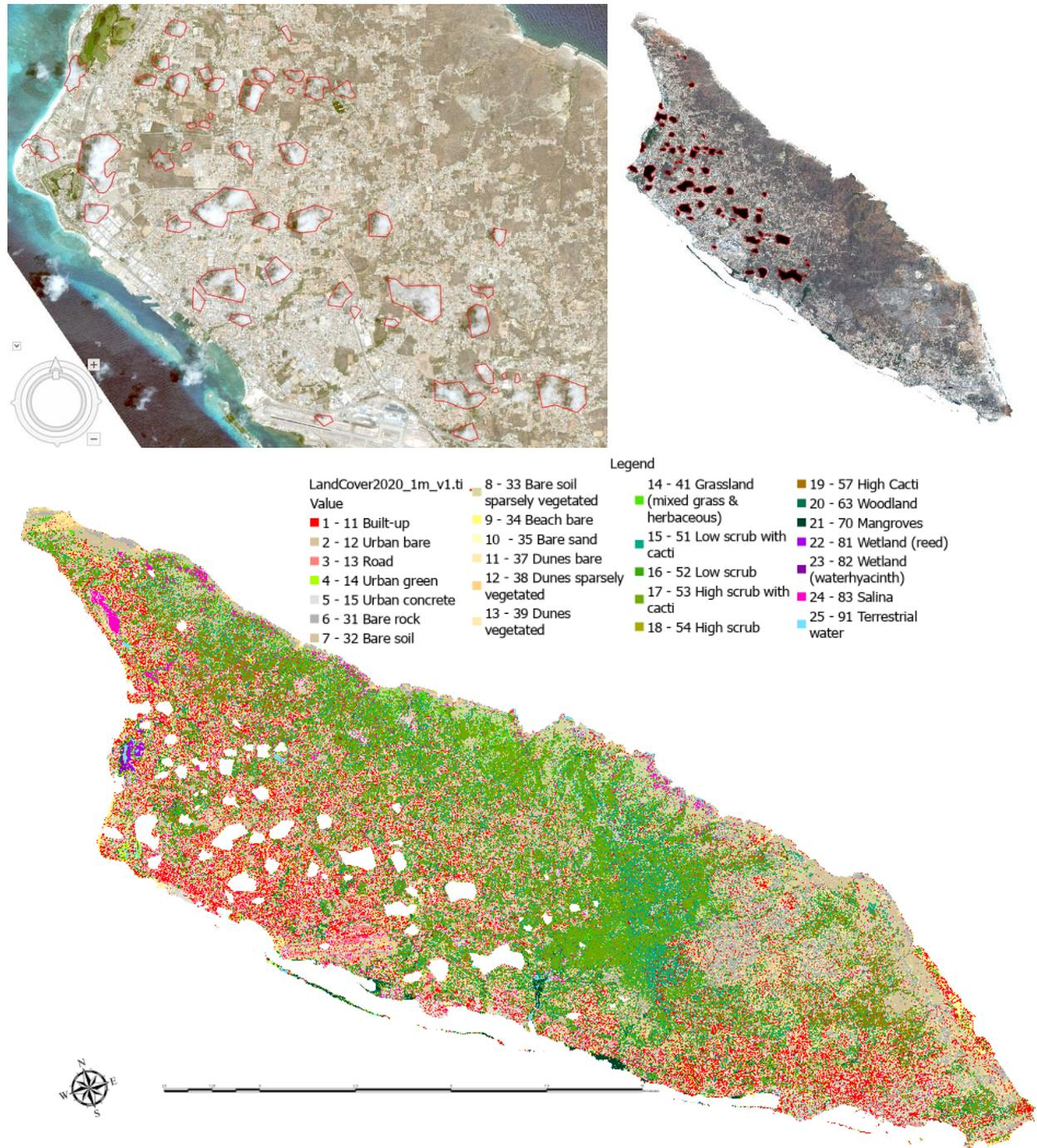
**Figure 8** Visual identification of clouds (left), the resulting eight-band multispectral mosaic at 1.2 m resolution (mosaic\_Aruba\_WV3\_2020\_MS8b.tif) and the result of the maximum likelihood classification.
