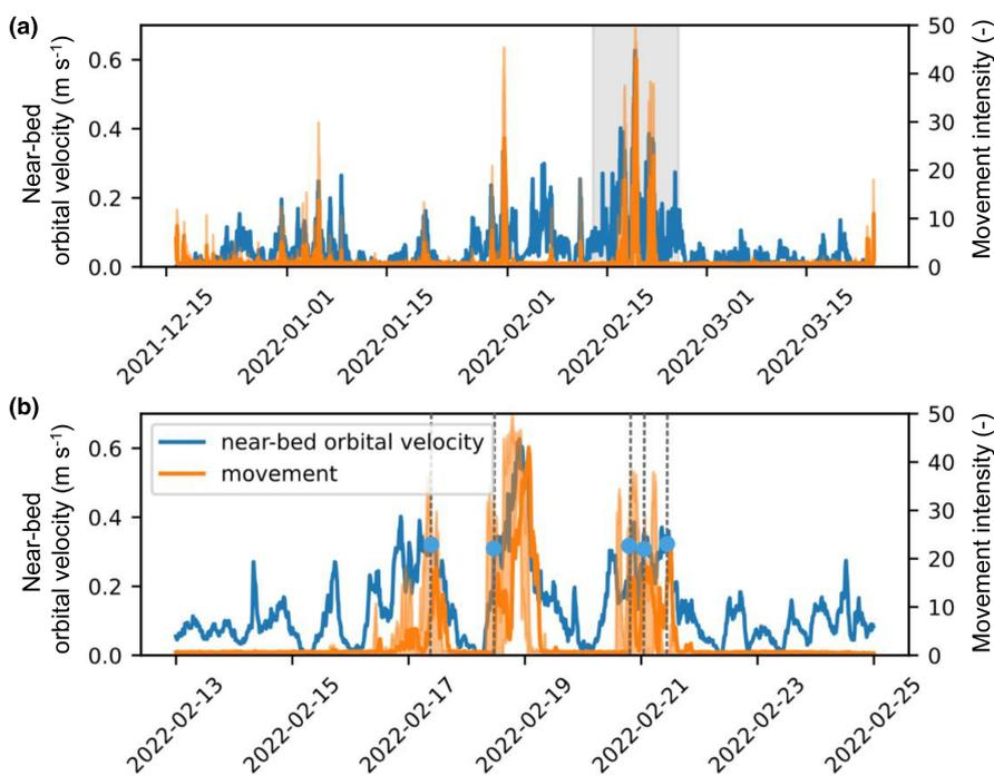
**FIGURE 3** (a) Near-bed orbital velocity and mean movement intensity of the aggregated MCAs (Mussel Clump Accelerometer; developed to quantify mussel clump movement) during field monitoring period, with the storm period outlined in grey. (b) Near-bed orbital velocity and mean MCAs movement intensity during the storm period. Vertical dashed lines and blue markers indicate MCAs dislodgement events.
