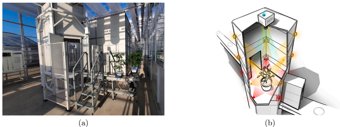
Fig. 3. The imaging system - Maxi-Marvin - being used to acquire individual plant point cloud data. (a) shows the outline of the imaging unit; (b) shows a schematic drawing of the camera setup inside the imaging black box.
