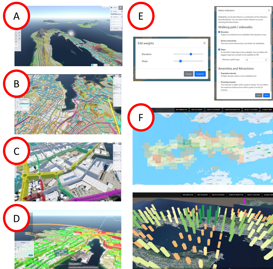
FIGURE 9. Digital twin for mobility design. A: 3D scene navigation; B: Demography specification; C: Road network design; D: Traffic simulation; E: Walkability parameter definition; F: Walkability 2D/3D visualization.
