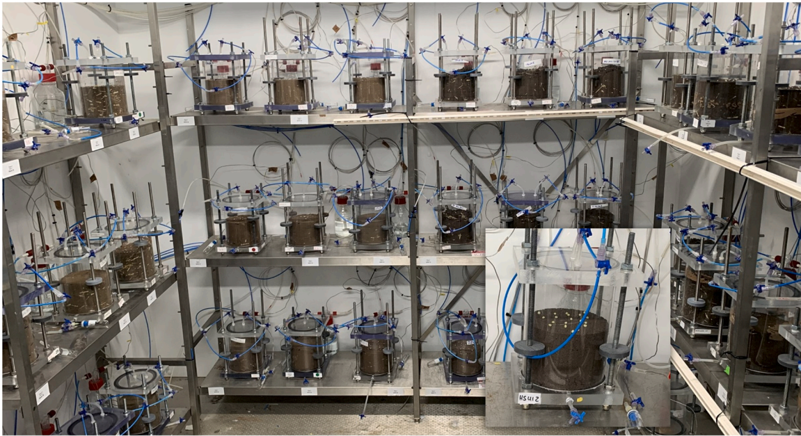
Fig. 1. Set-up of flow chambers for N 2 O quantification.
