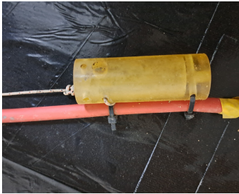
Figure 3.6: Star oddi casing, attached to cord of heater with spacing of one meter from each oddi
