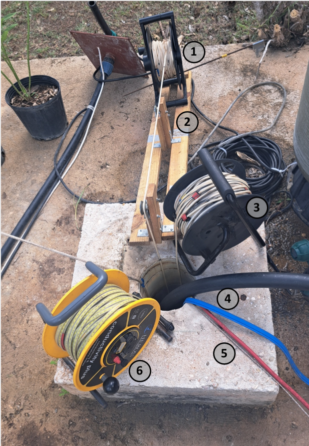
Figure 3.2: Set up of pump test with tracer measurements. With the numbers depicting: 1) rope reel CTD (Conductivity Temperature Depth) logger 2) pulley system 3) rope reel diver 4) pump tube and electrical cord 5) cord heater and oddi line 6) dipper
