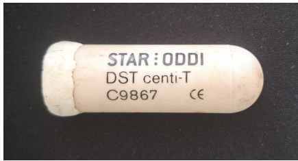
Figure 3.5: Star oddi, Temperature measuring device
