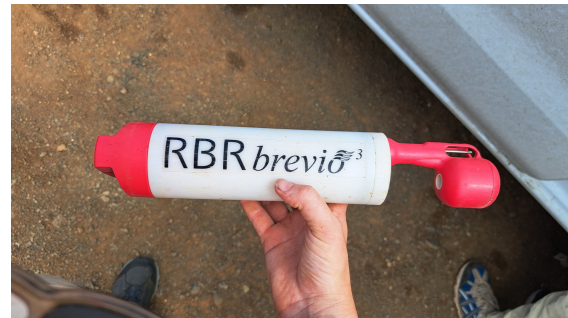
Figure 3.4: The used CTD-logger, it is a RBR Brevio 3
