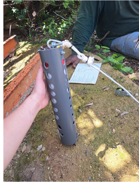
Figure 3.3: Casing used around the CTD-logger to protect from potential damage made to the RBR Brevio by the well wall
