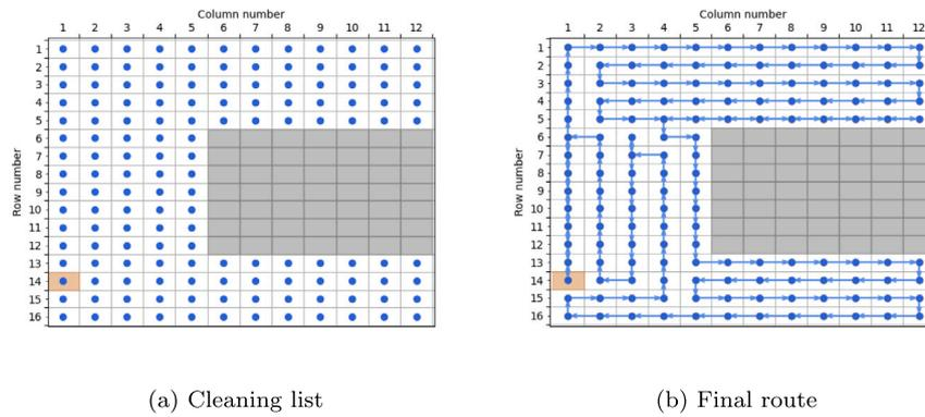
Fig. 7. Scenario 1: Fixed routes, (a) grids to clean (blue dots), and (b) the programmed route (blue arrows connecting the dots) and both graphs show the start grid (orange fill).
