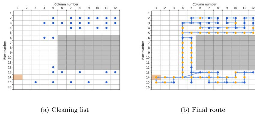
Fig. 8. Scenario 3: cleaning approach using grid-based RL, (a) grids to clean (blue dots), and (b) the programmed route (blue arrows connecting the blue dots). In addition the grids visited, but not on cleaning list (orange dots) and both graphs show the start grid (orange fill).
