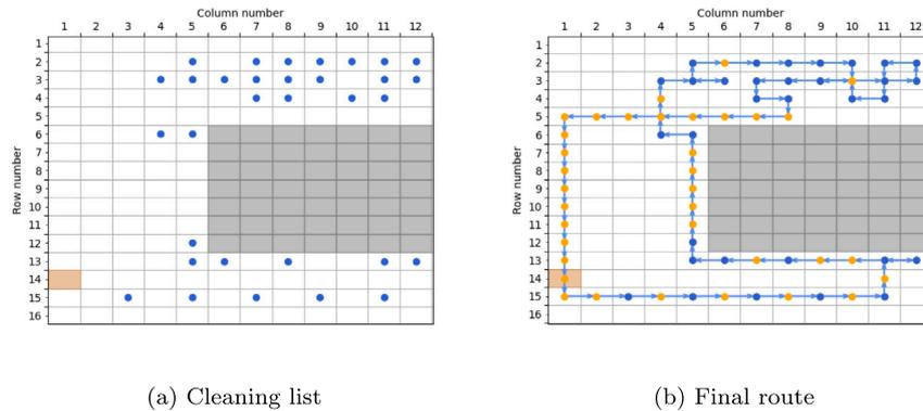
Fig. 9. Scenario 4: ideal routes produced by simulated annealing for TSP, (a) grids to clean (blue dots), and (b) the programmed route (blue arrows connecting the blue dots). In addition the grids visited, but not on cleaning list (orange dots) and both graphs show the start grid (orange fill).
