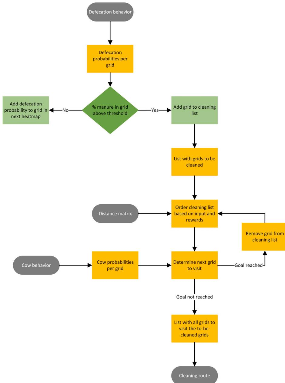
Fig. 4. Flowchart of the cleaning procedure. Rectangles indicate processes, diamonds indicate decisions and round shapes indicate inputs/outputs.
