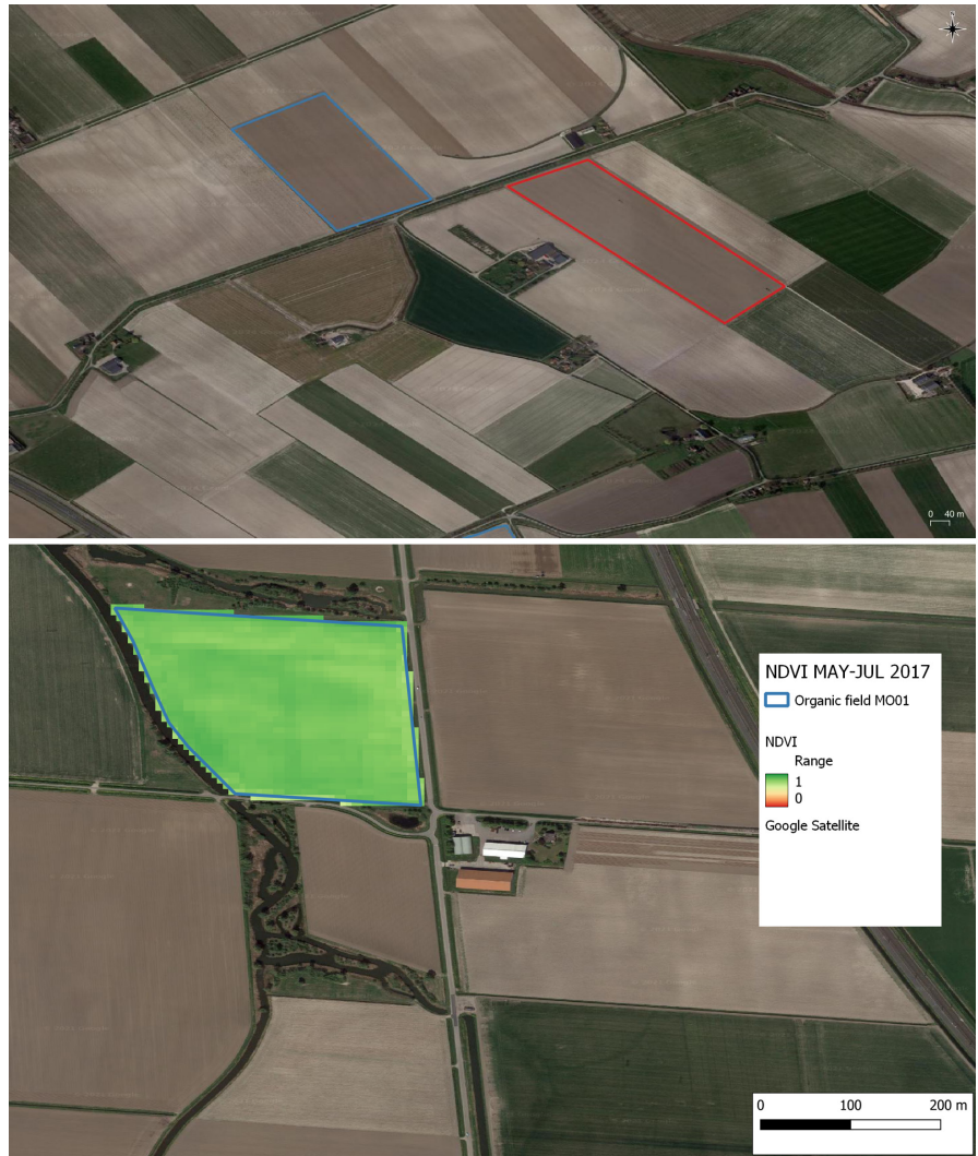
FIGURE 1 Example of organic farm field paired with field from nearby conventional farm. Images were acquired from the Sentinel-2 satellite and processed in Google Earth Engine to obtain NDVI. Red polygon: conventional farm, blue polygon: organic farm. Green color represents greenness (NDVI). NDVI, normalized difference vegetation index.
