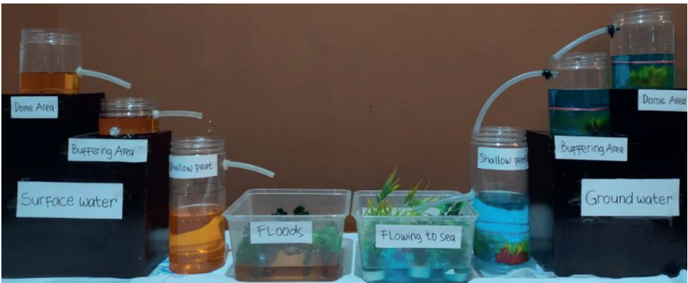
Figure 5D.3. Simple water balance model of H 2 Ours game in Pawan-Kepulu peatland to show the dynamics of changes in hydrological conditions because of the changes in land-use and canal density. The red line in each tank in the groundwater system represent the fire vulnerable threshold.
