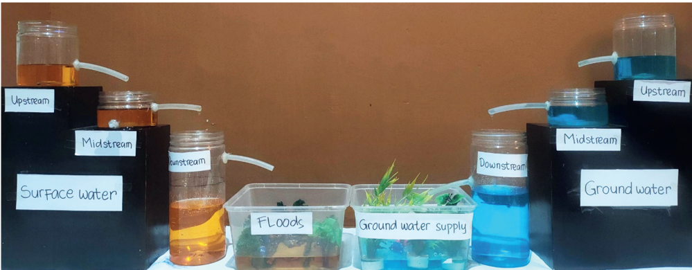
Figure 5.6. Simple water balance model of H 2 Ours game in the Rejoso watershed to show the dynamics of changes in hydrological conditions because of land-use change and water utilization. See Appendix 5D for the simple water balance model for the Pawan-Kepulu peatland.
