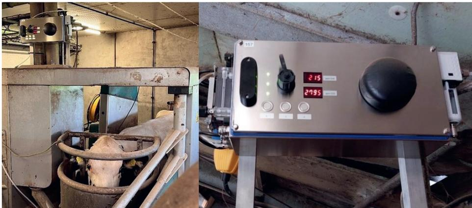
**Figure 1.4.** The sniffers as used for phenotyping methane emissions for this thesis. A cow standing in an automated milking system (AMS), where breath is sampled from the feed bin, the sniffer is installed near the AMS at the top left (*left*). The sniffer records a value of 215 ppm methane and 2,795 ppm carbon dioxide (*right*)
