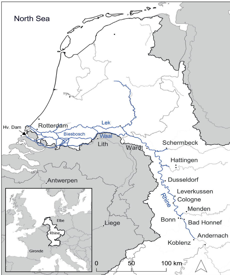
Figure 3.1. Map overview of the study area. In white: the delta and lower river part of the Rhine river basin. In blue: three combined SOBEK models (see Table 3.1), whereby modelling of the Rhine was done for the Netherlands and the German state of North Rhine-Westphalia (from the North Sea until Bad Honnef). Hv. Dam = Haringvliet Dam.
