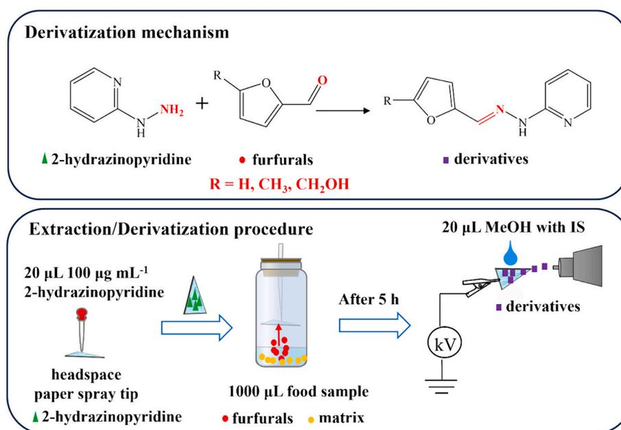
**Fig. 1.** (A) Overview of the derivatization reaction. (B) Schematic diagram of the HSPS-MS/MS procedure. 2-Hydrazinopyridine was dropped on a paper tip and dried. Furfurals entered the headspace from the food sample and were derivatized on the paper. Finally, the paper was analyzed by PS-MS/MS.
