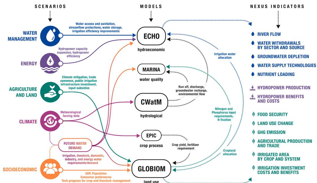
Fig. 3. Schematic overview of the integrated nexus modelling framework (INMF) for the Zambezi River Basin. Source: Authors' own elaboration; Graphic Design: Adam Islaam
