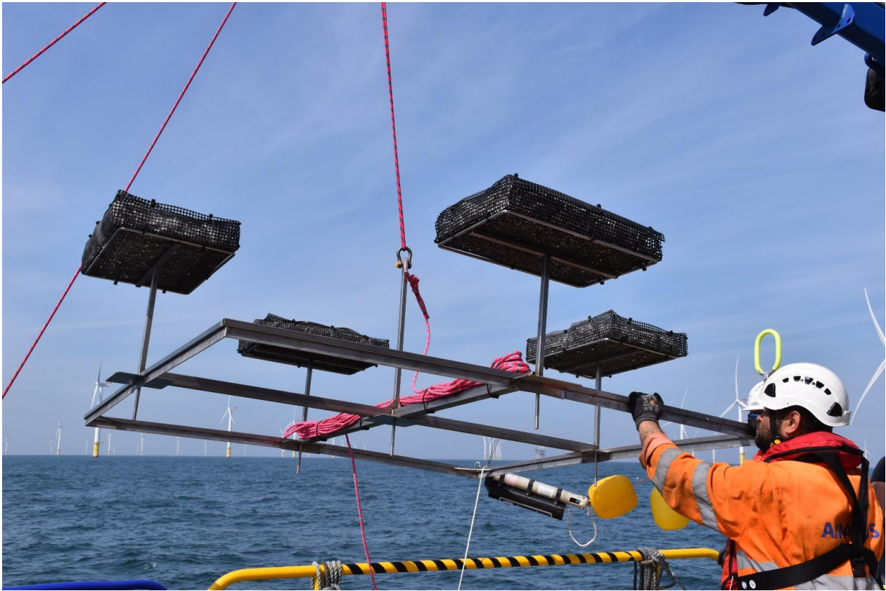
Figure 6. Deployment of oyster spat collector (photo: Renate Olie, DRN).
